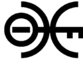
Wi-Fi with closed SSID
